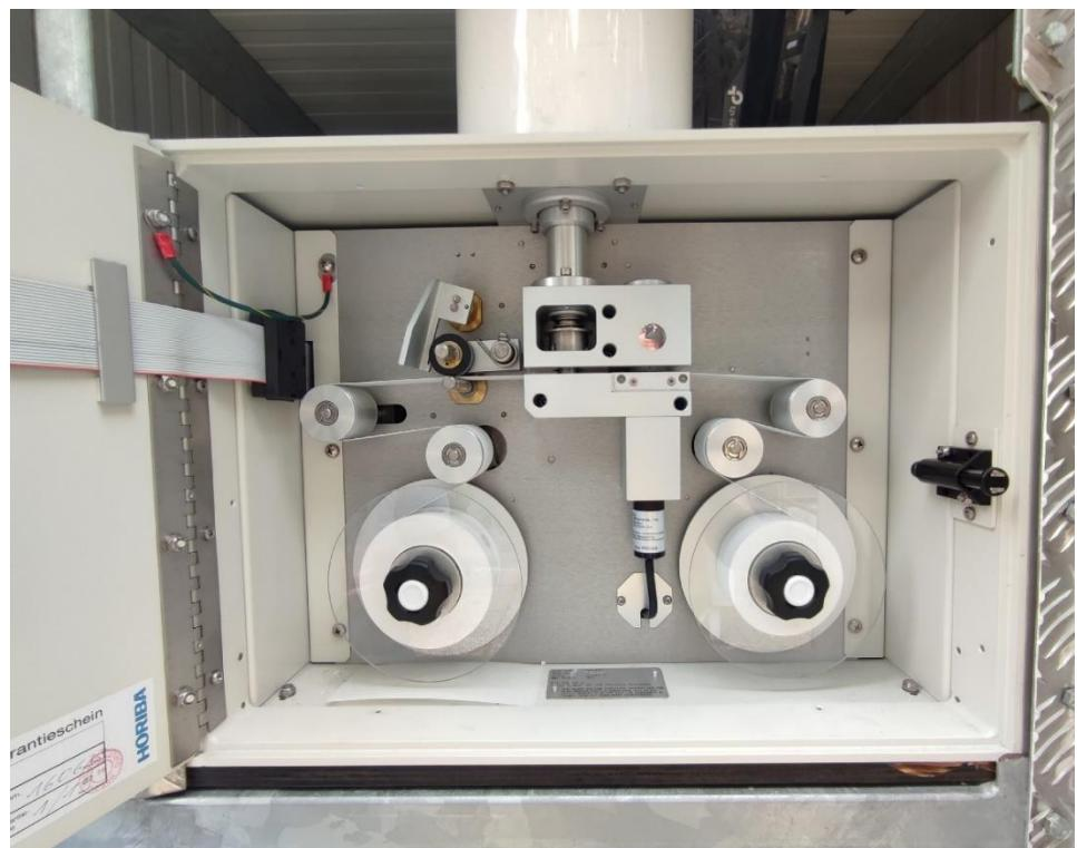
**Slika 11.** Filterske trake u analizatoru Horiba APDA – 371
