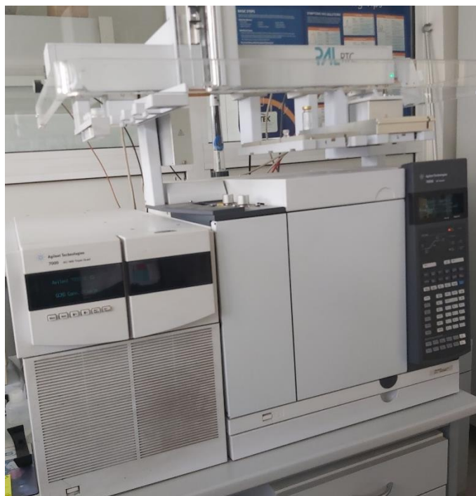
Slika 2. „GC-MS/MS Agilent 7000, GC/MS triple quad, GC 7890b“
