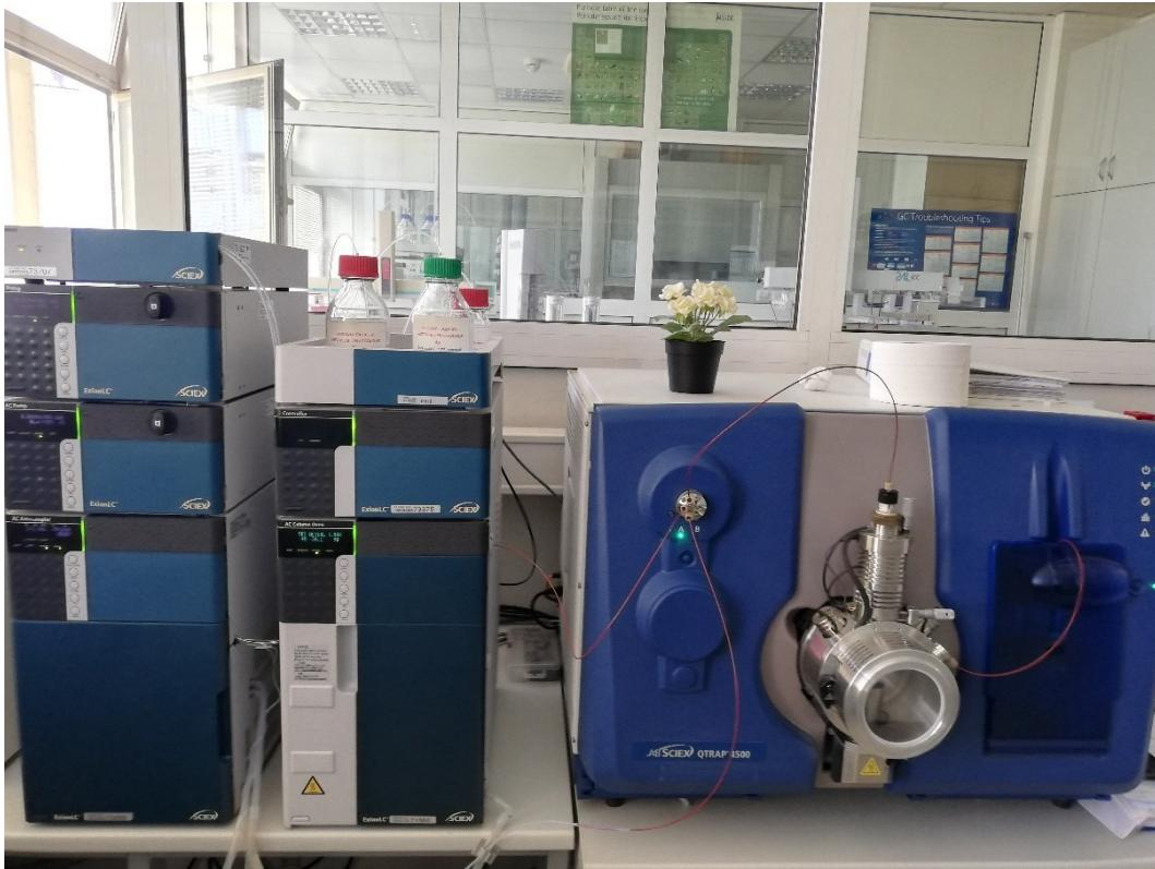
**Slika 9.** LC-MS/MS Sciex Triple Quad™ 4500, HPLC Sciex ExionLC
