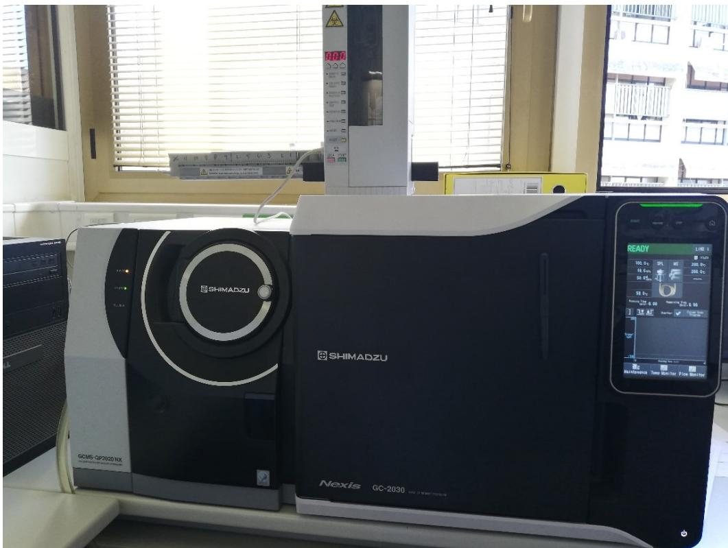
**Slika 11.** GC-MS Shimadzu GC/MS-QP 2020 NX, NEXIS GC 2030
