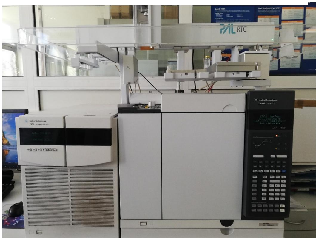
**Slika 10.** GC-MS Agilent 7000 Series Triple Quad
