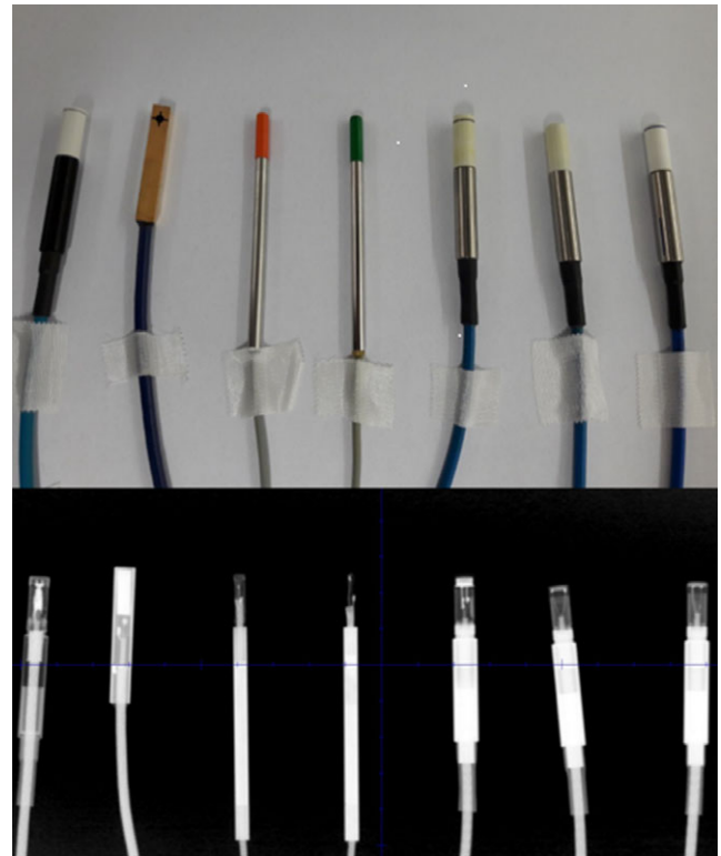
Fig. 1. Photo (top) and x-ray image (bottom) of six diodes and microdiamond detector used in this study. From left to right: PTW 60019 mD, SN EDGE Detector, IBA Razor diode, IBA SFD diode, PTW 60008 Diode P, PTW 60012 Diode E, and PTW 60018 Diode SRS. [Color figure can be viewed at wileyonlinelibrary.com ]
