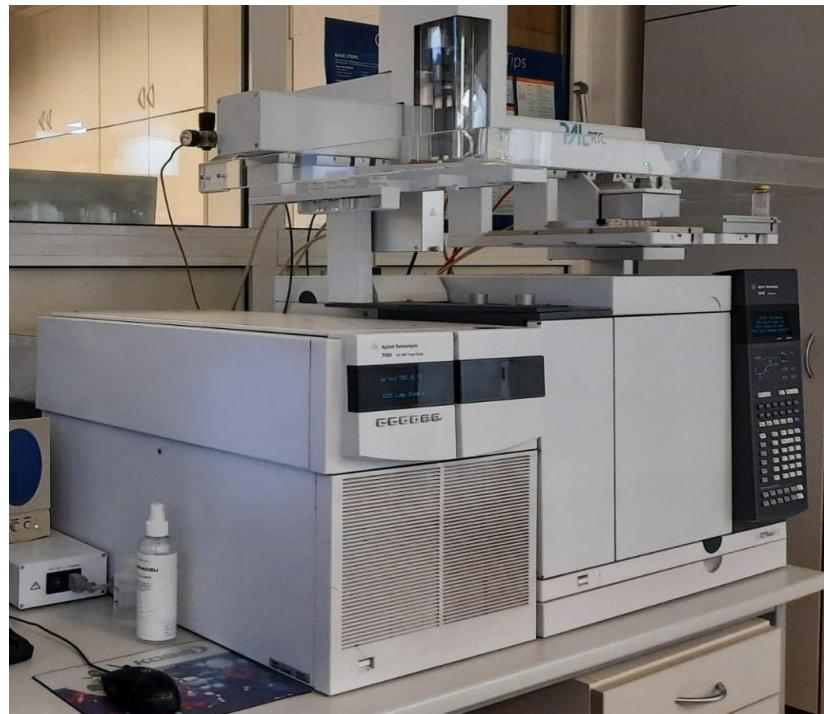
Slika 8. GC-MS/MS Agilent 7000, GC/MS triple quad, GC 7890b
