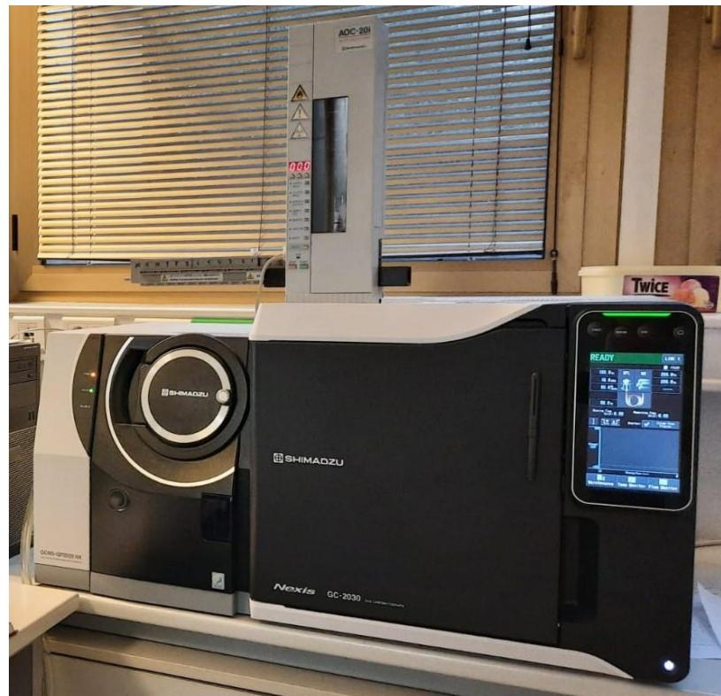
Slika 9. GC-MS Shimadzu, GCMS-qp 2020 nx, GC GC-2030 nexionis
