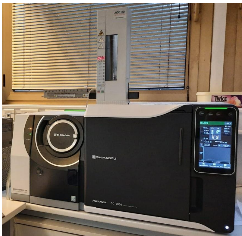
Slika 9. GC-MS Shimadzu, GCMS-qp 2020 nx, GC GC-2030 nexis
