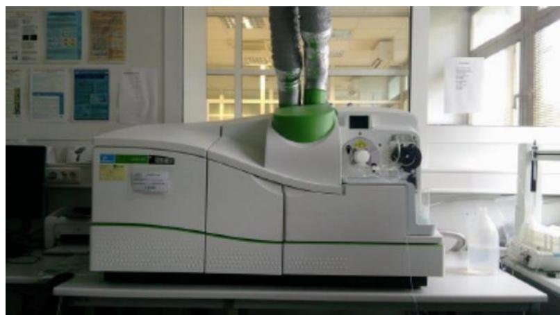
**Slika 5.** ICP-MS NexION 300x Perkin Elmer
