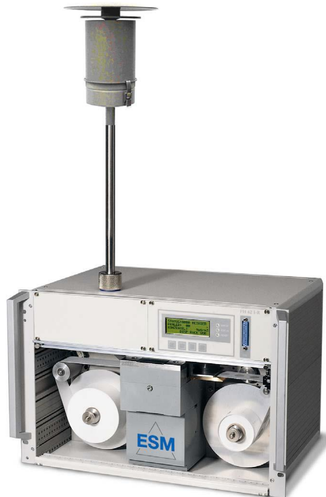
Slika 9. Instrument za monitoring \text{PM}_{10} , FH 62 I-R
