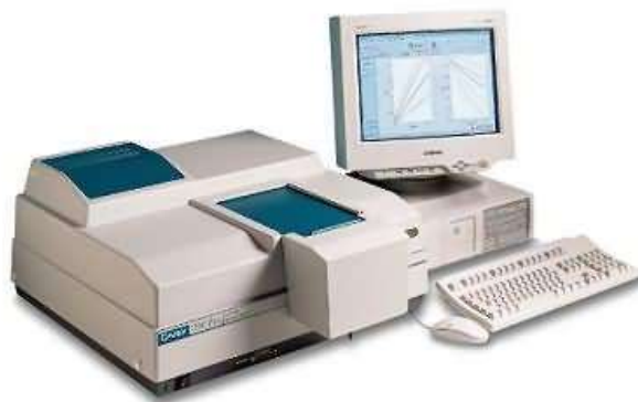
Slika 9. Spektrofotometar, Cary 100 Bio WINUV, UV-Visible, Varian, Australija (preuzeto s: http://www.speciation.net/Database/Instruments/Varian-Inc/Cary-100-UVVis-spectrophotometer-;i379 )
