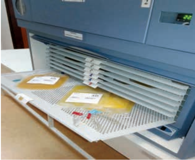
Figure 2. Platelet incubator with agitator
