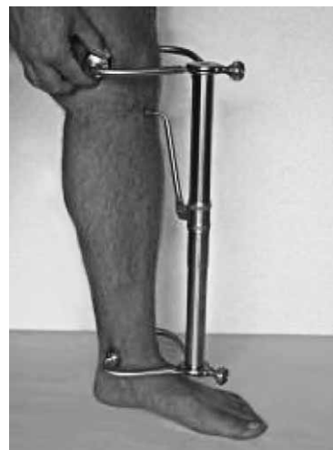
Fig. 2. Torsionmeter in use.
