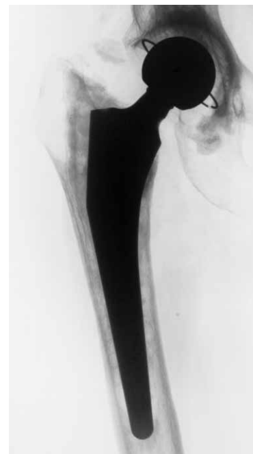
Fig. 1. X-ray of the Müller type cemented hip prosthesis with a stem occupying <90% of femoral canal diameter: A – directly after implantation; B – loosened 5 years later.
