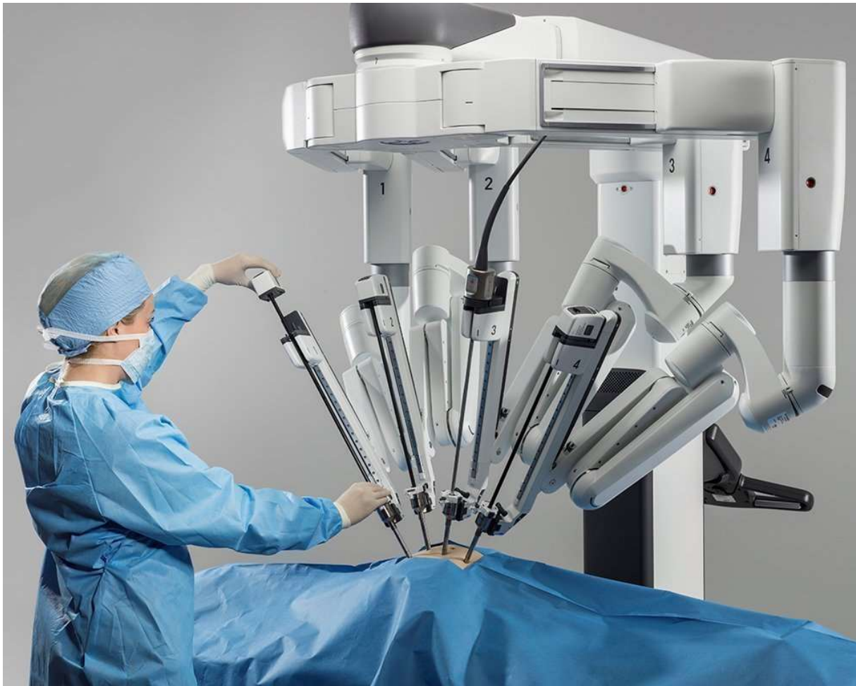
Slika 12. Da Vinci robotski sutav, (preuzeto s https://aimis.com/robotics/about-us/davinci-xi )
