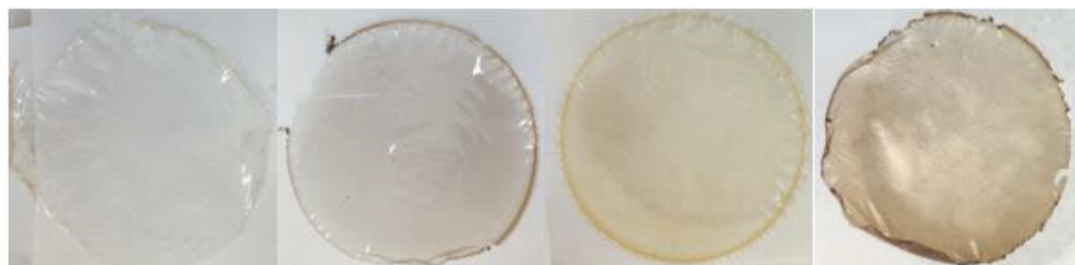
Figure 3. Picture of produced films (from left to right, CSGEL, CSGELGA, CSGELOEO, CSGELGAOEO). CSGEL—chitosan/gelatin; GA—gallic acid; OEO—orange essential oil.
