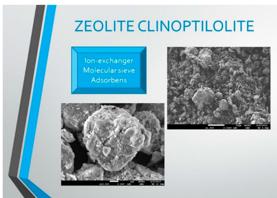
Figure 5. Electron micrographs of zeolite particles that can serve as ion exchangers, molecular sieves as well as an adsorbent. Images were obtained by SEM Jeol JSM-7800F.
