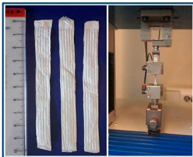
Figure 2. Tensile testing of the electrospun scaffolds.
