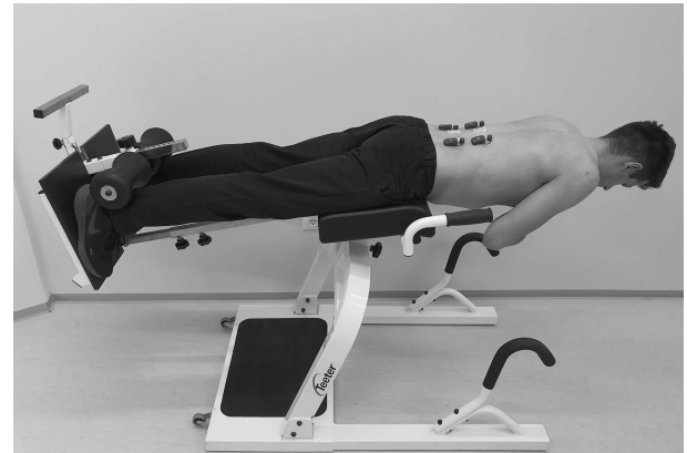
FIGURE 1. Tilting device in the Roman chair configuration used for testing with the subject placed in the trunk extension position.
