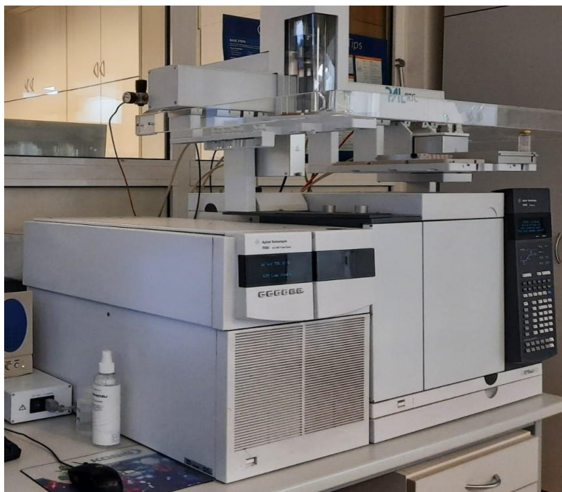
Slika 8. GC-MS/MS Agilent 7000, GC/MS triple quad, GC 7890b
