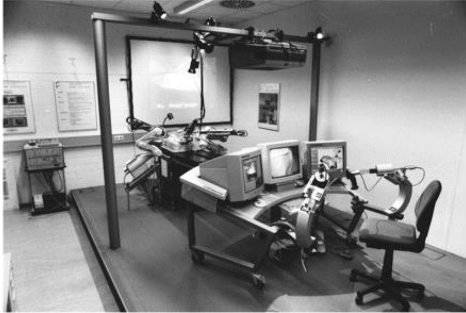
Slika 1. ARTEMIS – Advanced Robotic Telem manipulator for Minimally Invasive Surgery.
