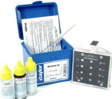
Slika 17. Test DPD (izvor: <https://www.poolvacparts.com/taylor-chlorine-dpd-midget-test-kit.html?cmp=bingshopping&kw=taylor-chlorine-dpd-midget-test-kit>)
