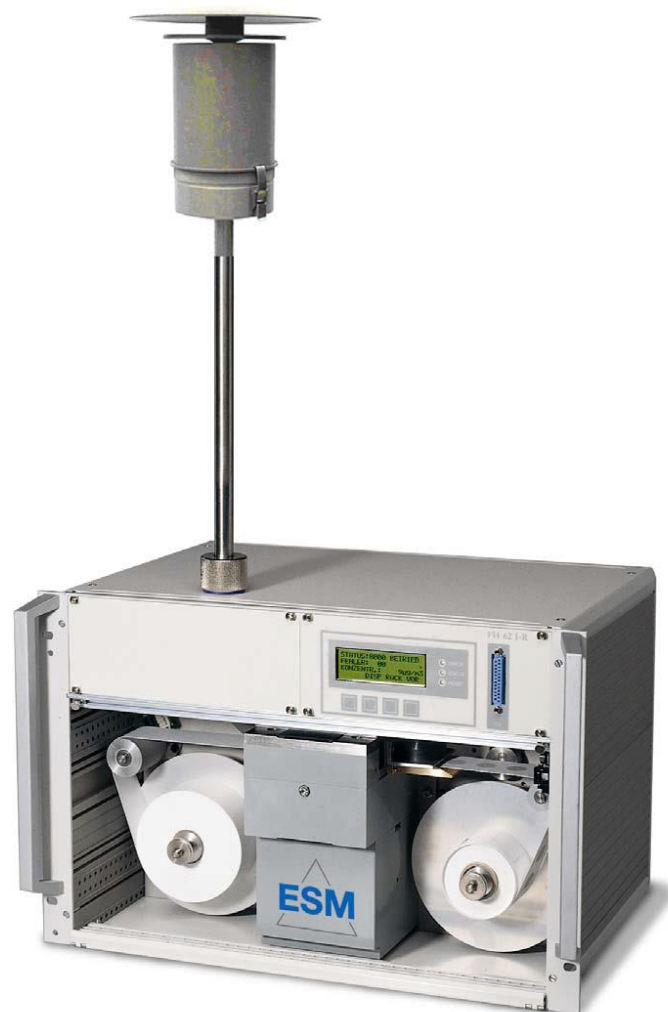
Slika 9. Instrument za monitoring \text{PM}_{10} , FH 62 I-R
