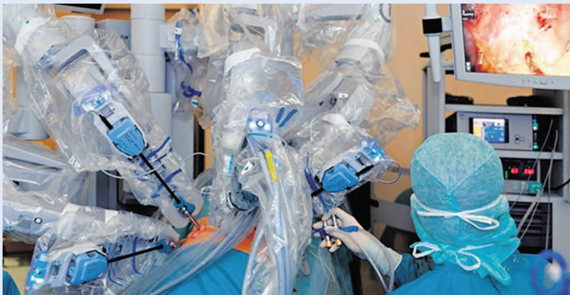
Figure 1. Robotic system da Vinci Si® Surgical System (Intuitive Surgical, USA) during surgery (with permission from the personal archive of Prof. Berlakovich).
