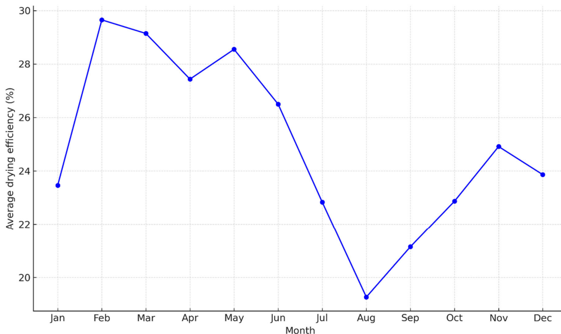
Figure 5. Monthly variation in average drying efficiency (%). The plot illustrates the average drying efficiency for each month, highlighting seasonal trends in the biodrying process. Data points represent the mean drying efficiency calculated across all observations within each month.
