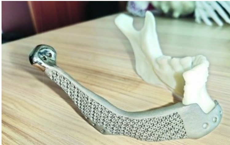
Slika 6. Primjer modela parcijalnog mandibularnog implantanta proizvedenog od titanija uz pomoć DMLS aditivne tehnologije (33). (Preuzeto iz: Hosnti.com. Application of 3D Printing Titanium and Titanium Alloy in Repair of Jaw Defect; Dostupno na: https://www.hosnti.com/2019/08/28/application-of-3d-printing-titanium-and-titanium-alloy-in-repair-of-jaw-defect )
