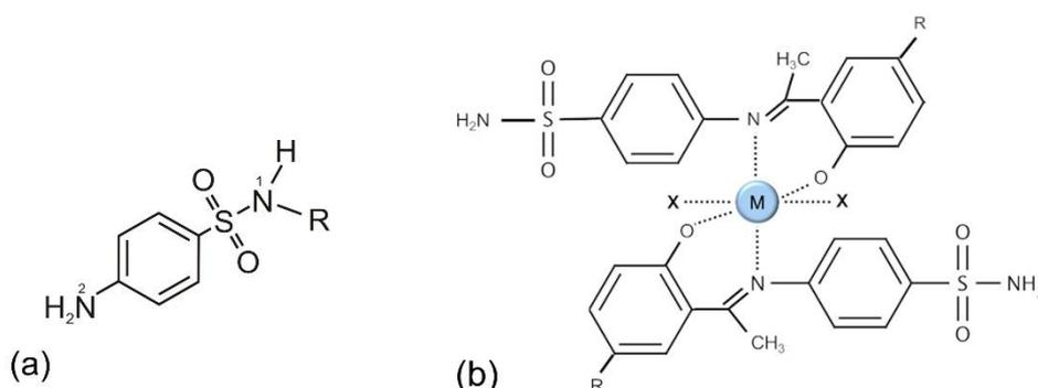
**Figure 6.** (a) General structure of sulfonamides. (b) Chelation is not relevant in the classical sulfonamide mode of action, but the chelates of new-generation sulfonamide molecules with metal (M) cations (M = Co<sup>2+</sup>, Ni<sup>2+</sup>, Cu<sup>2+</sup>, Zn<sup>2+</sup>, and VO<sup>2+</sup>) demonstrate antibacterial and antioxidative activities; inspired by ref. [49].
