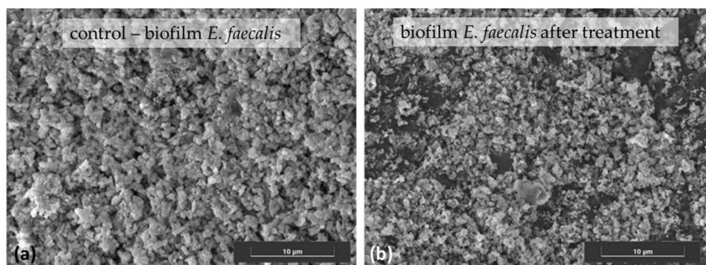
**Figure 2.** SEM images of *E. faecalis* on urinary catheter surface (a) before and (b) after nitroxoline treatment, showing the areas of biofilm destruction. Samples were coated with Pd before analysis on a Hitachi S–3600N Scanning Electron Microscope. Image taken at 13.3 k magnification (scale bar represents 10 µm).
