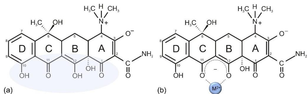
**Figure 3.** (a) Structure of tetracycline. The shaded area emphasizes the part relevant for chelating ability. (b) An example of a simple tetracycline–Mg chelate.
