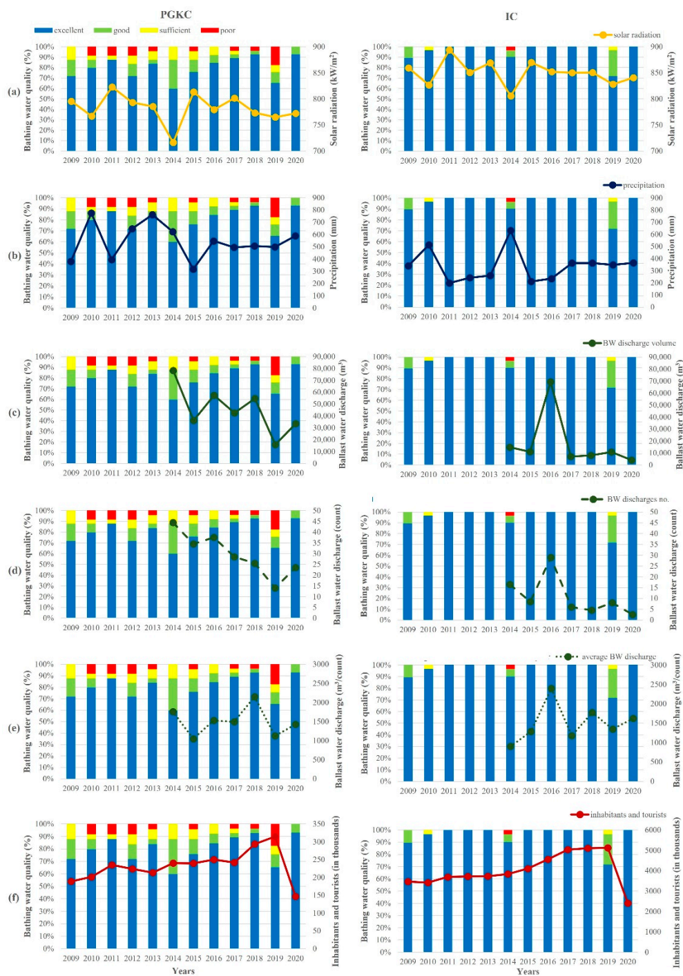
Figure 8. Yearly averages of the bathing water quality in the surrounding area of the port of Rijeka (PGKC; left) and the port of Pula (IC; right) with cumulative values of (a) solar radiation, (b) precipitation, (c) total BW discharge, (d) number of BW discharges, (e) ratio between total BW discharge and number of discharges and (f) number of inhabitants and tourists. Calculations were based on values obtained during bathing seasons (from mid-May to late September) over the 12-year period (2009–2020).
