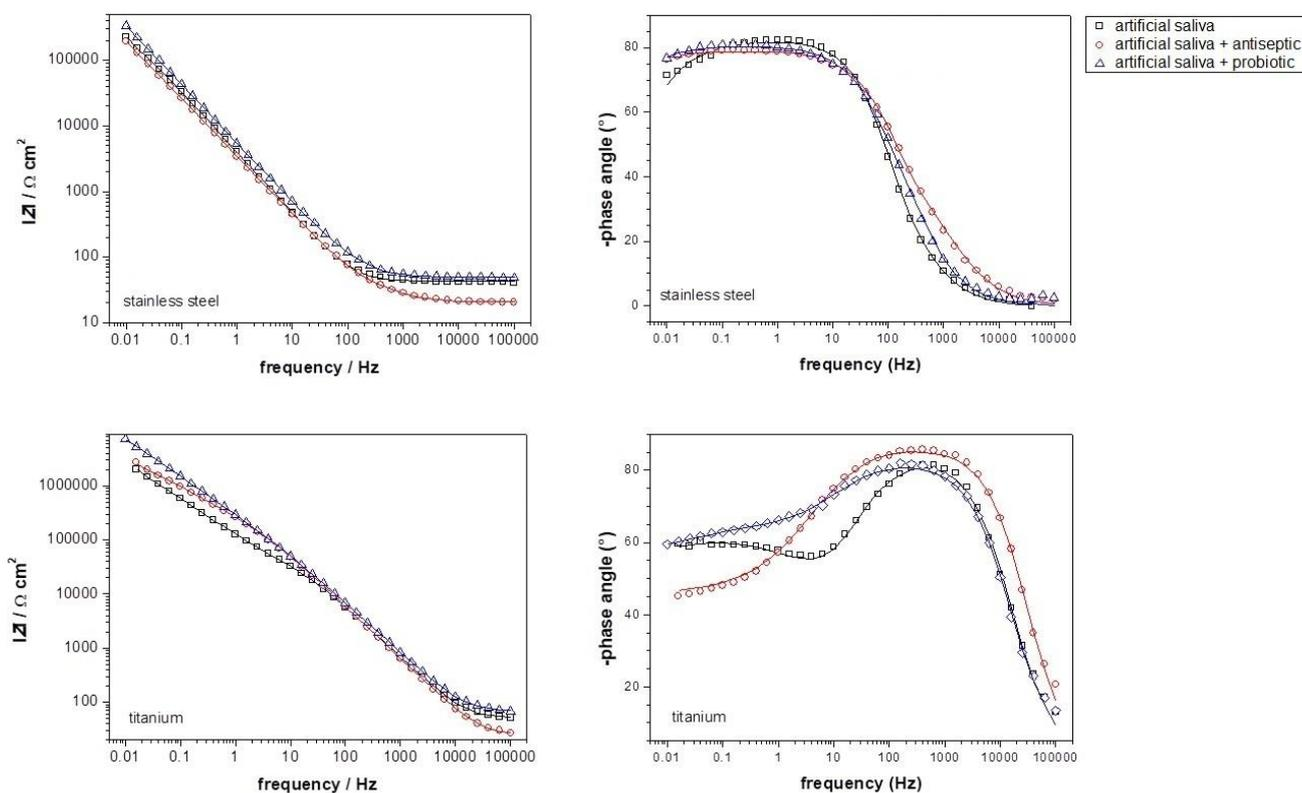
**Figure 2.** Electrochemical impedance spectra for stainless steel and titanium mini implants exposed to artificial saliva, oral antiseptic and probiotic supplement. Symbols represent measured and lines fitted data. The y-axis presents the impedance module (left figure) and phase angle (right figure), while the x-axis presents the excitation frequency.
