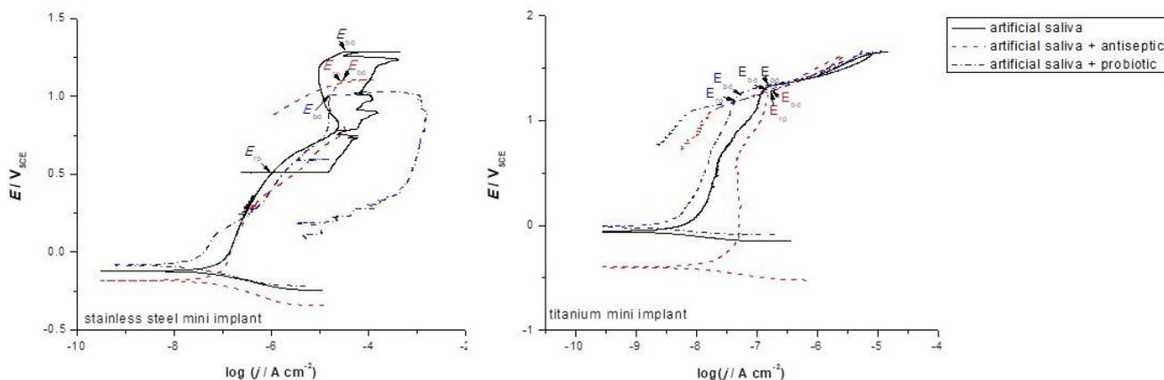
**Figure 1.** Cyclic polarization curves of stainless steel and titanium mini implants exposed to artificial saliva and oral antiseptic and probiotic supplements. The x-axis represents the current density ( $j$ ), and the y-axis represents the difference between the working electrode and counter electrode potential ( $E$ ).
