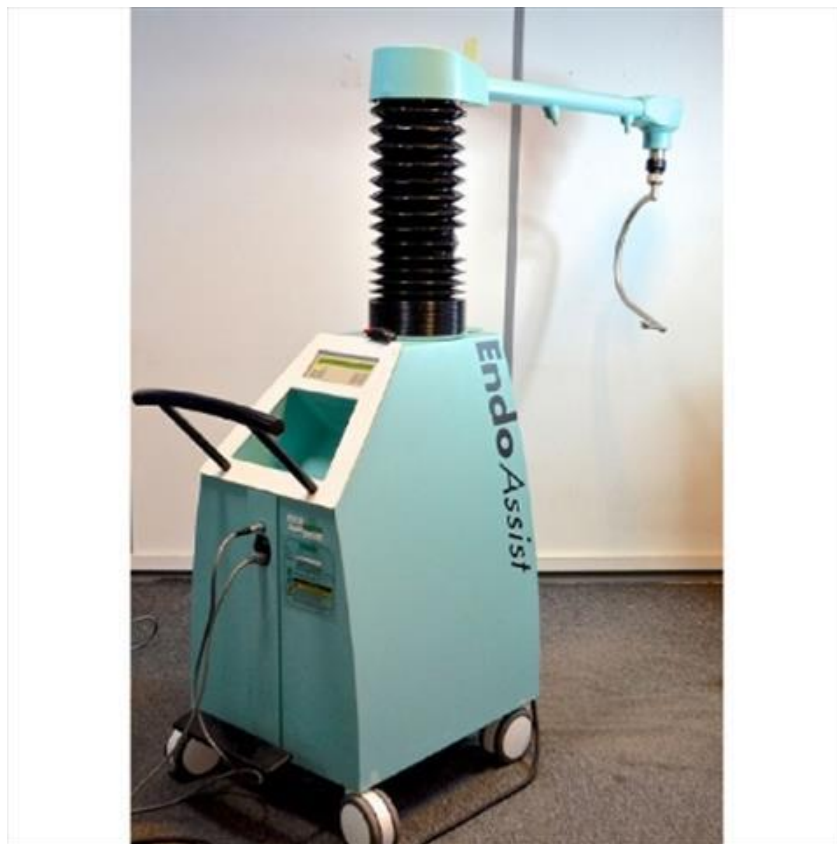
Slika 5. Endoassist robotski sustav (preuzeto s https://hilditchgroup.com/lotimages/H881C1-79-0 3.8.2021)
