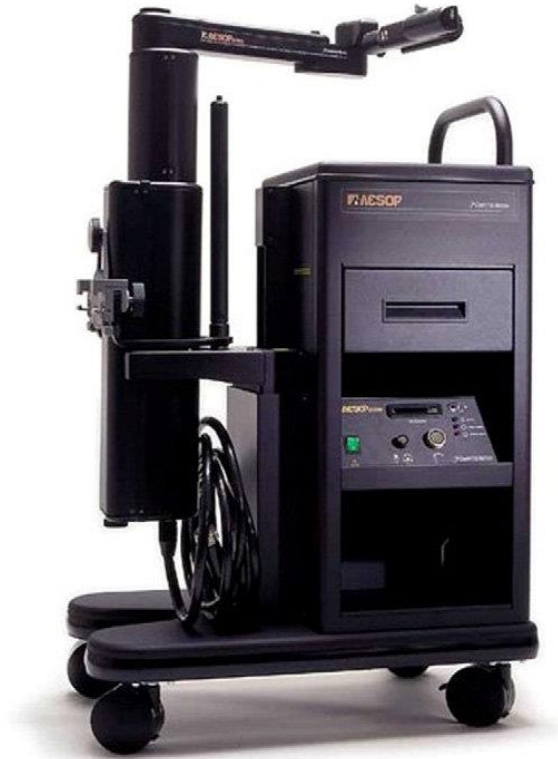
Slika 4. Computer Motion AESOP - Kirurški robotski sustav (preuzeto s https://www.researchgate.net/profile/Robert-Holloway-3/publication/51437277/figure/fig2/AS:610718843928576@1522618127649/Computer-Motions-AESOP-Automatic-Endoscopic-System-for-Optimal-Positioning-has-allowed . 3.8.2021)
