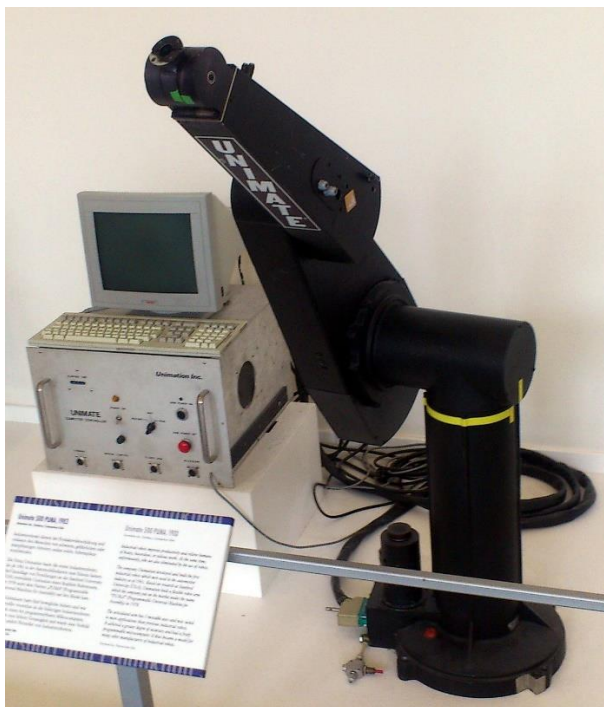
Slika 2. PUMA – Programmable Universal Machine for Assembly (preuzeto s https://upload.wikimedia.org/wikipedia/commons/thumb/b/b8/Unimate_500_PUMA_Deutsches_Museum.jpg/1200px-Unimate_500_PUMA_Deutsches_Museum 27.7.2021)
