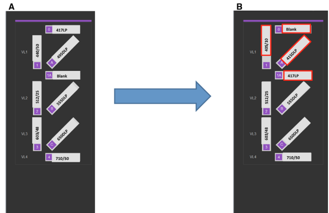
Figure 75. Use of the Attune NxT No-Wash No-Lyse Filter Kit. The standard configuration for the 405 nm violet laser optical filter block is shown in (A) and the same optical filter block using the No-Wash No-Lyse Filter Kit shown in (B), with changes outlined in red. To use the filter kit, remove the 440/50 bandpass filter in VL1 slot 1 and place the 405/10 bandpass filter that is placed in the VL1 slot 1in slot 1. Remove the 495 Dichroic Longpass (DLP) filter in a lot A the 415DLP. The Blank filter in slot 1A is switched with the 417LP filter in slot 0.
