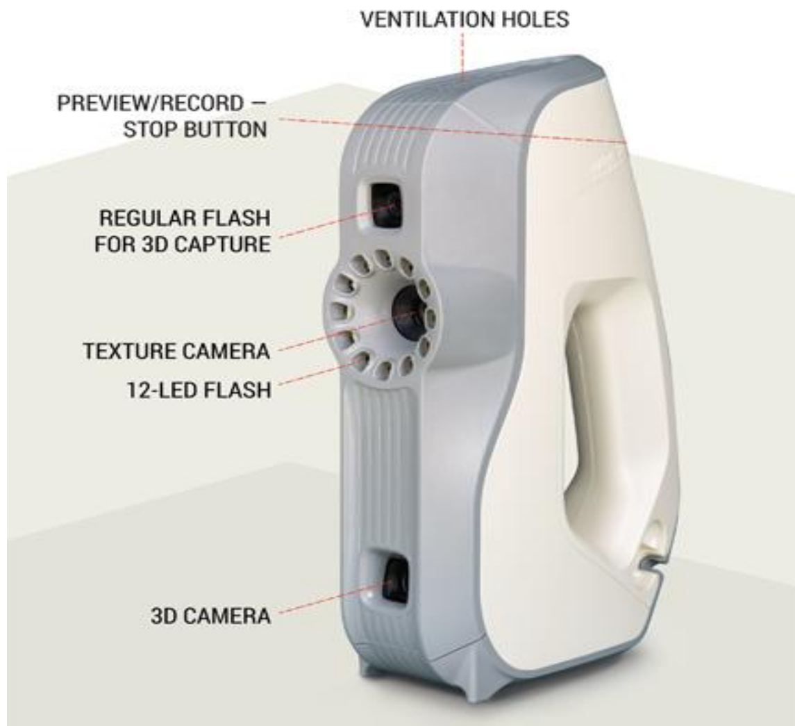
Figure 10: Structured light 3D scanner Artec Eva Available from: http://docs.artec-group.com/as/11/en/hardware.html [cited 2018 Jun 15].
